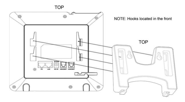
Figure 3: GXP16xx Wall Mount installation
